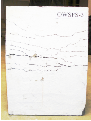
Fig. 5. Crack pattern of specimen with SR=21
