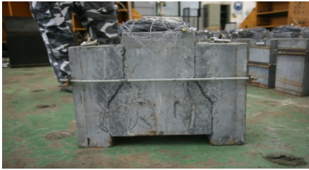
Fig. 8. Failure of UHPFRC precast joint (Cast-in-place joint)
