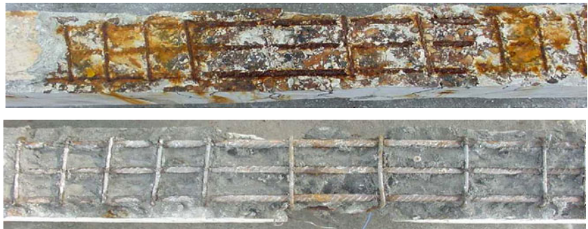
Fig. 8. Corrosion status of steel in OPCC-2 beam (Top) and FGC-3 beam (bottom)
